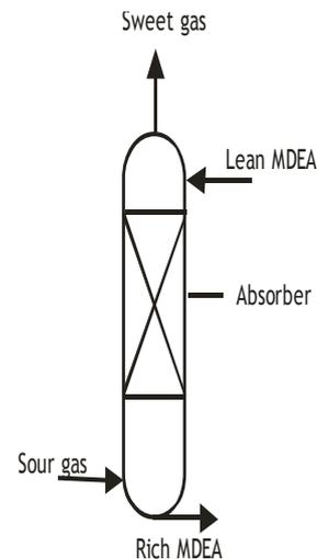
Figure 1: Schematic of the Absorber
