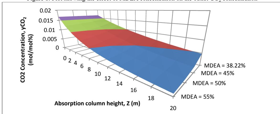
Figure 9: Surface plot of CO<sub>2</sub> concentration along column height at varying concentrations of MDEA
