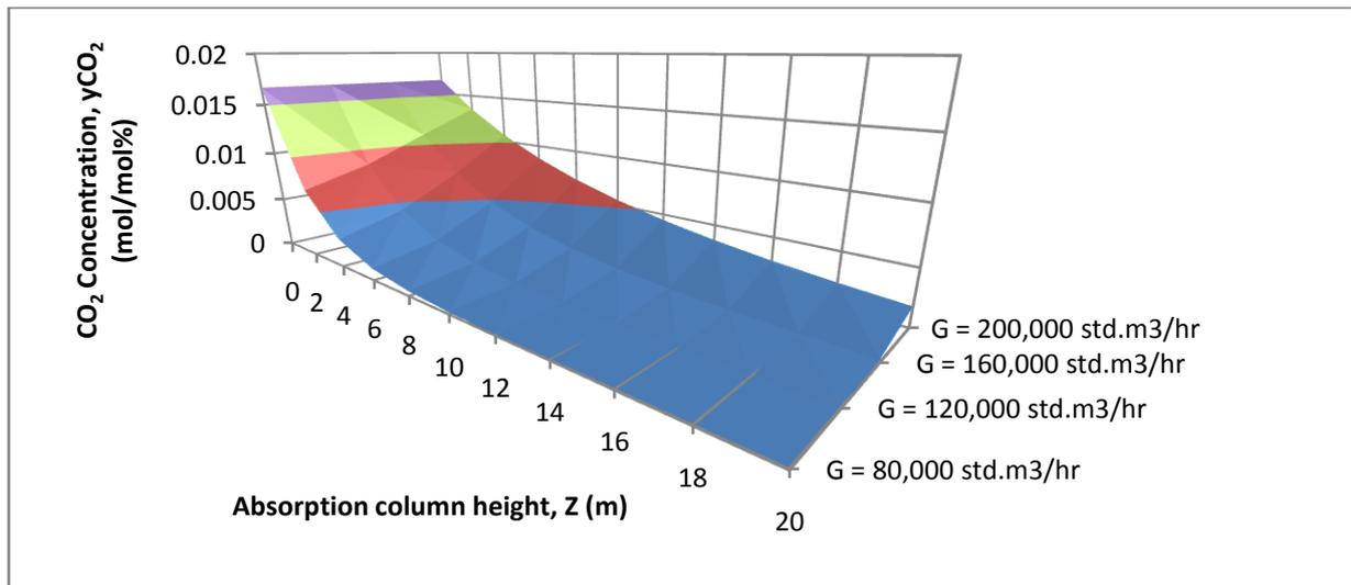
Figure6: Surface plot of CO<sub>2</sub> concentration through column height at different gas flow rates
