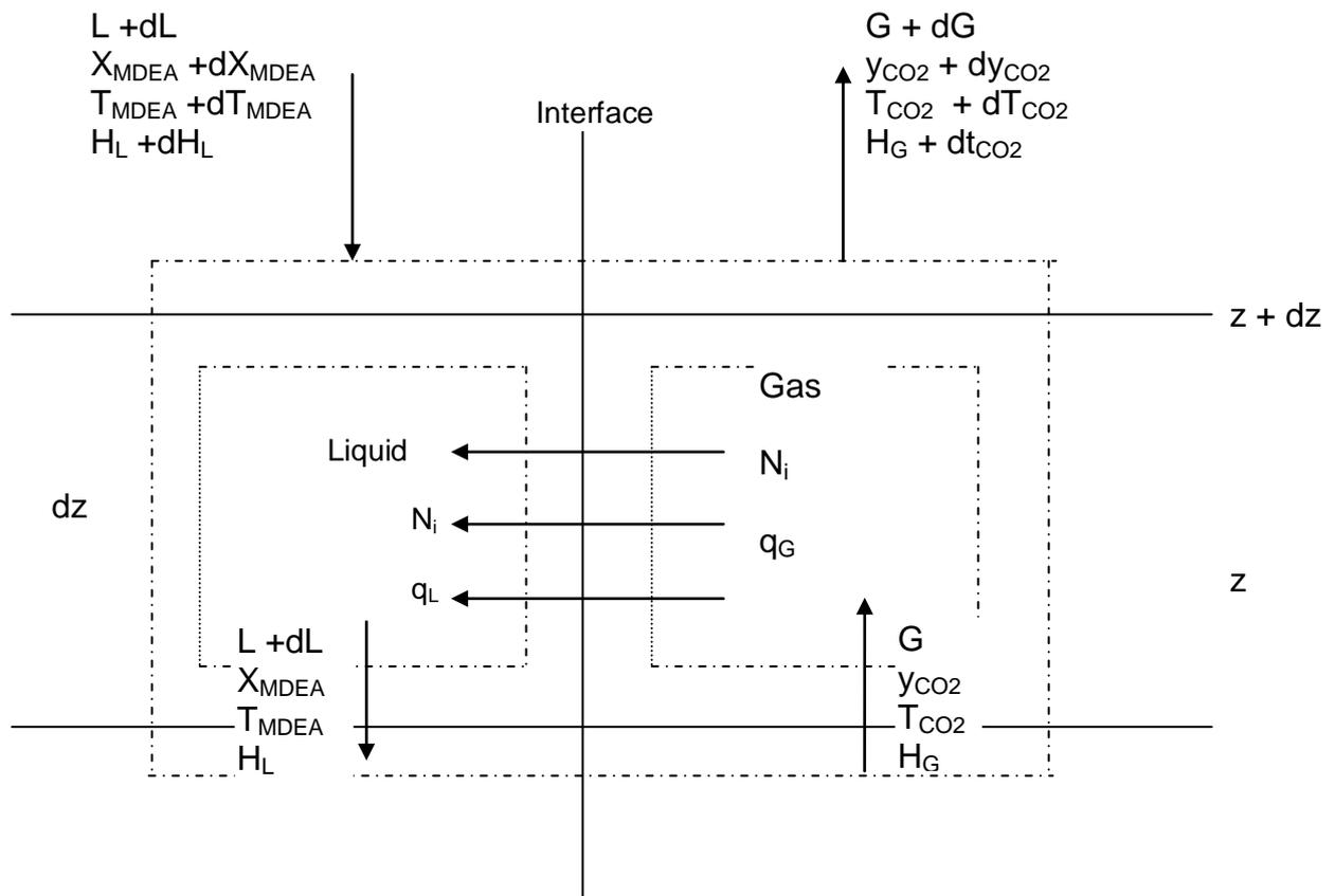
Figure 2: Mass and heat transfer in differential section of the Absorber
