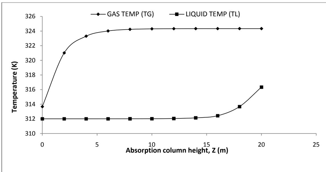
Figure 4: Gas and Liquid stream temperatures along the absorption column height.
