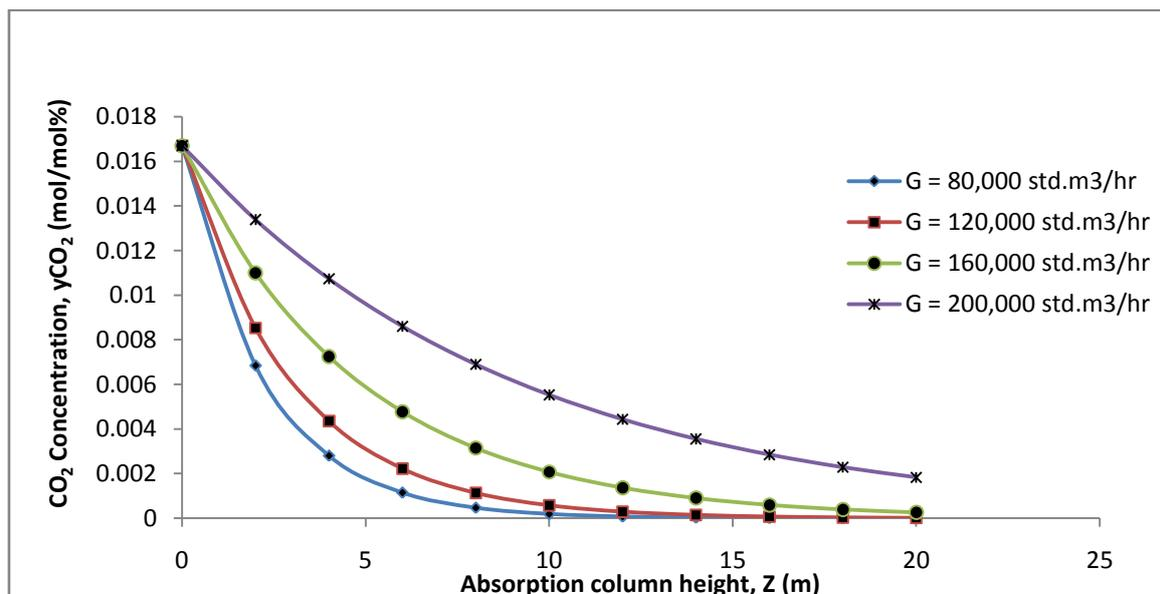
Figure 5: Carbon dioxide concentration along column height for different gas flow rates.
