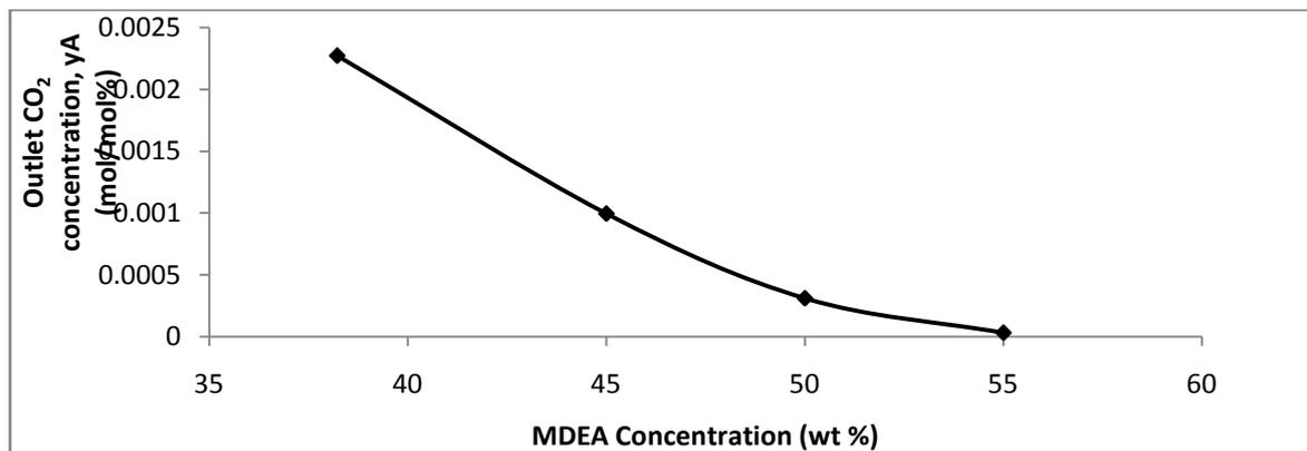
Figure 8: Plot showing the effect of MDEA concentration on the outlet CO<sub>2</sub> concentration
