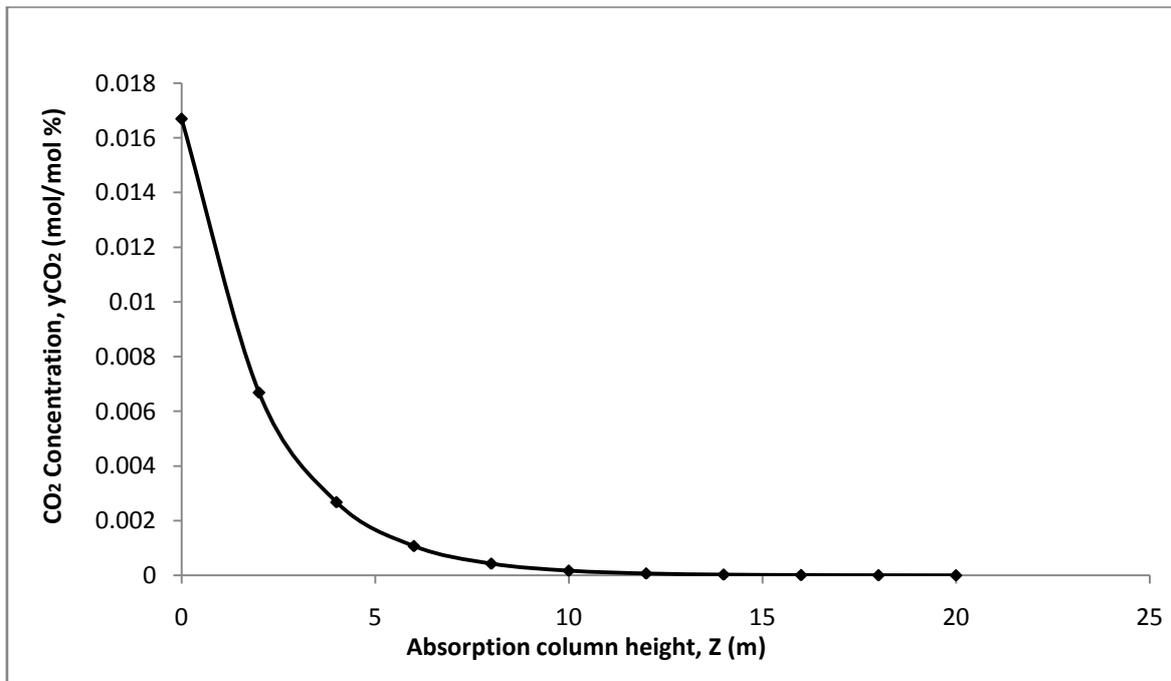
Figure3: Variation of gas CO<sub>2</sub> concentration(mole fraction) from bottom of column
