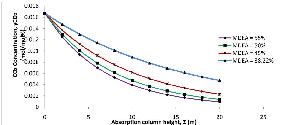
Figure 7: Effect of concentration of MDEA on carbon dioxide concentration
